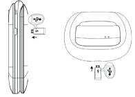
1. Insert the charger connector into the phone. 2. Connect the charger to a power outlet.
